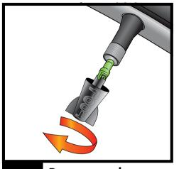
Remove valve core with included tool.
